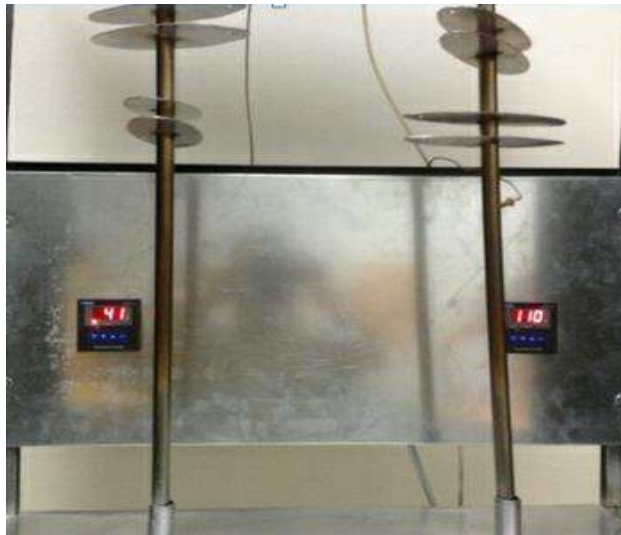
Figure 1. Elliptical fin shape at different axis used in the experimental work for natural convection
