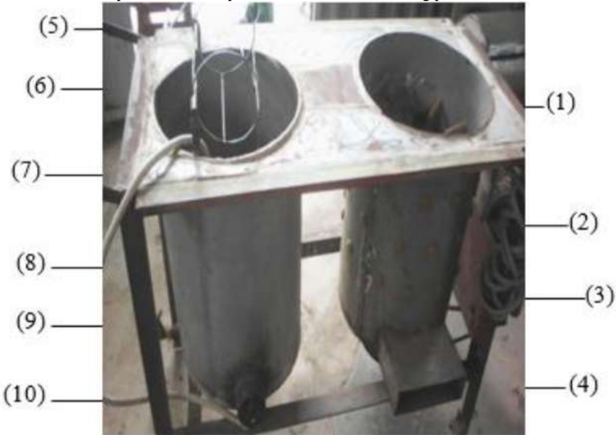
Figure 2 The fabricated de-feathering machine with scalding tank.
