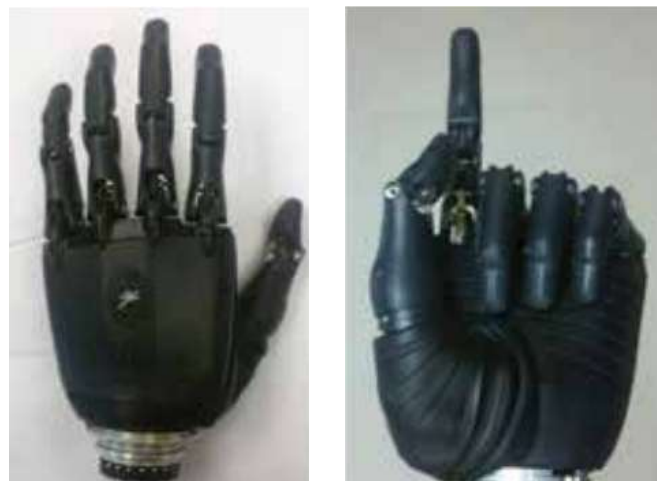
Figure 9. BeBionic hand Examples of different grip patterns possible [10].
