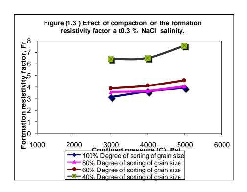
These data demonstrate that for the same amount of grain sorting, the formation resistivity factor grows by raising the pressure. A decrease in the electric current path caused by an increase in the confined pressure The formation resistance factor accordingly rises. which produces a rise in Both the extent of sorting
