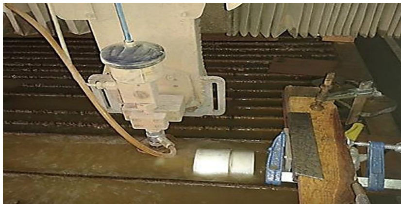
Fig. 3. Submerged abrasive water jet experimental setup.
