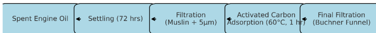
Figure 2: Simplified process flow for the recycling of spent engine oil using settling, filtration, and activated carbon adsorption. The method emphasizes low-cost, low-energy treatment stages suitable for decentralized oil recovery.
