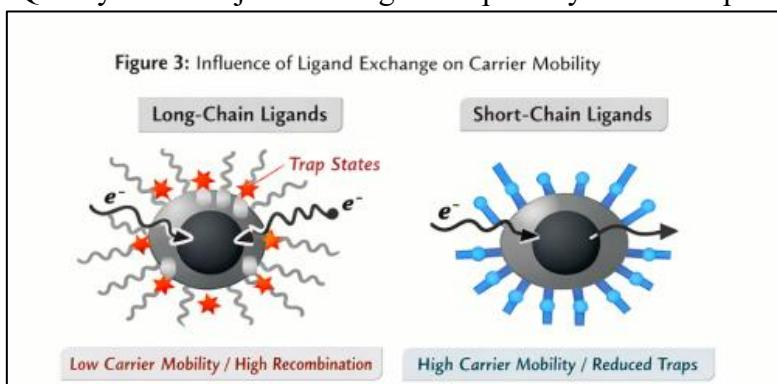
conduction and valence band edges can be tuned through halide composition and ligand chemistry, allowing PQDs to function either as primary absorbers or as interfacial layers that improve carrier extraction and reduce recombination (Yang et al., 2023).
