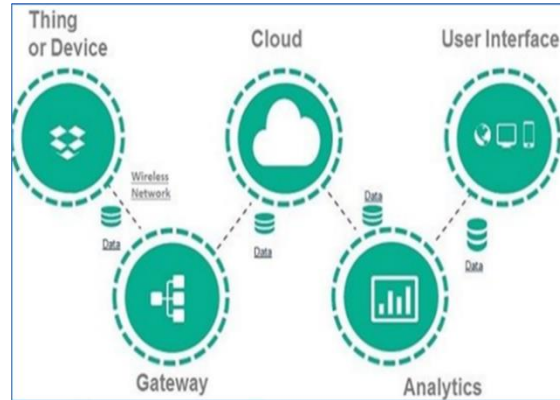
FIGURE (2) MAIN COMPONENT ELEMENTS OF THE INTERNET OF THINGS
